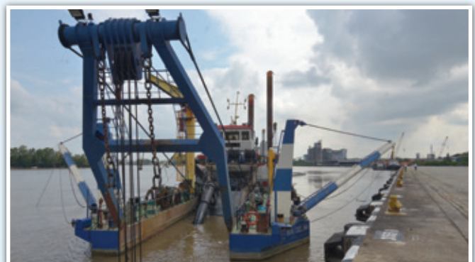
Penyelenggaraan pengerukan dermaga di Terminal Senari dan Pending. Maintenance dredging alongside wharves at Senari and Pending Terminal.
